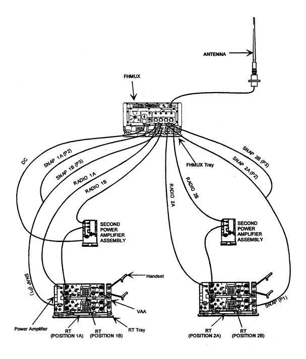
Figure 5-4. Cable Diagram: For TD-1456/VRC
